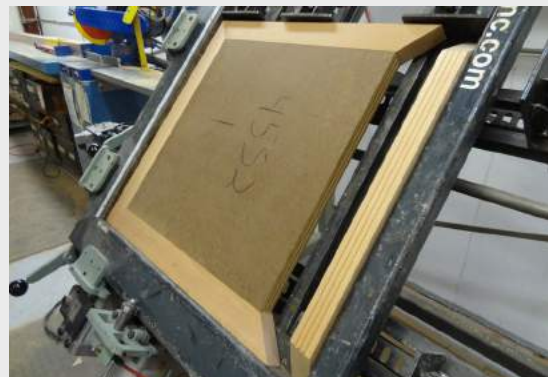
Rim Raised Panel Construction
