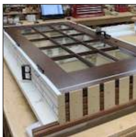
The sill is shimmed up 3/16" in the field to help water drain underneath the nose
